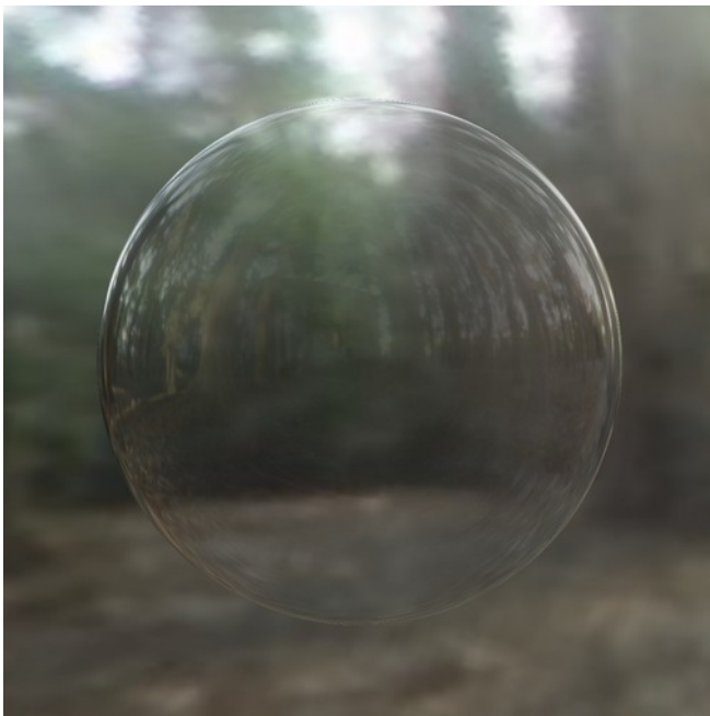
Figure 3. Hollow glass sphere viewed through a vertical linear polarizer (brightened to match original intensity). Reflection is reduced at top and bottom; transmission is reduced at left and right.
